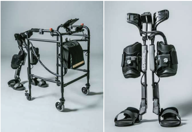
図2 装着型歩行支援ロボットWPAL (Wearable Power-Assist Locomotor)
